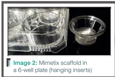
**Image 2:** Mimetix scaffold in a 6-well plate (hanging inserts)
