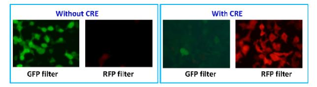
**Left panel / without CRE:** CRE reporter cell line (Cat#: **SC018-Bsd**) was created by LoxP460-Neo particles, cultured in 24-well-plate. Images were taken under microscope with GFP filter set (Ex 490nm/Em 525nm) and RFP filter set (Ex 545nm/Em 620nm).
