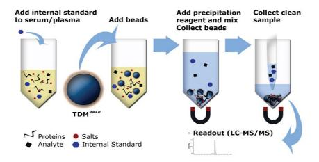
Sample preparation principle: In the first step the sample is lysed when whole blood is used and internal standard is added. The lysis step can be omitted when using serum. By addition of MagSiMUS-TDM<sup>PREP</sup> Type I Particle Mix and precipitation reagent proteins are bound to magnetic beads. The proteins are depleted from the reaction mix by simple magnetic separation. The purified sample can be directly injected into LC-MS/MS or can be stored for later analysis.
