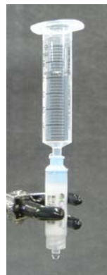
Picture 3. Syringe is directly connectable with Cellufine Mini-column.
