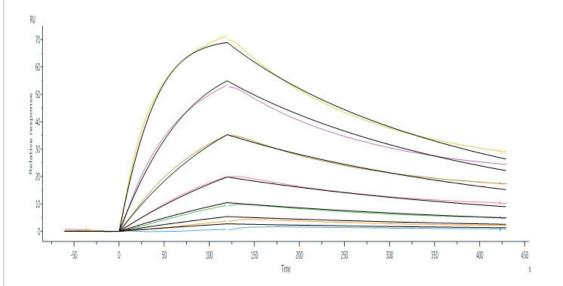
Biotinylated Human ACE2, His, Avitag (MALS verified) (Cat. No. AC2-H82E6) captured on Biotin CAP - Series S sensor Chip can bind 2019-nCoV Full Length S protein (R683A, R685A), His Tag (Cat. No. SPN-C52H4) with an affinity constant of 54.5 nM as determined in a SPR assay (Biacore 8K) (Routinely tested).
