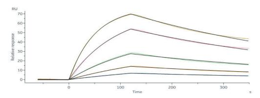
Biotinylated Human ACE2, His, Avitag (MALS verified) (Cat. No. AC2-H82E6) captured on Biotin CAP - Series S sensor Chip can bind 2019-nCoV S1 protein, His Tag (Cat. No. S1N-C52H3) with an affinity constant of 16.7 nM as determined in a SPR assay (Biacore 8K) (Routinely tested).
