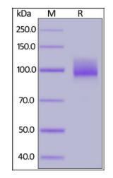
Biotinylated Human ACE2, His, Avitag (MALS verified) on SDS-PAGE under reducing (R) condition. The gel was stained overnight with Coomassie Blue. The purity of the protein is greater than 90%.
