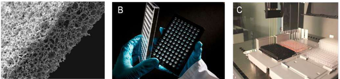
Figure 1: Alvetex® Scaffold 96-well plate: (A) Scanning electron micrograph showing the structure of an Alvetex® Scaffold membrane in cross-section. Note the highly porous architecture of the polystyrene-based material; (B) Alvetex® Scaffold 96-well plate product; (C) Automated robotic workstation housing an Alvetex® Scaffold 96-well plate with a multichannel pipette head enabling high throughput liquid handling capability.
