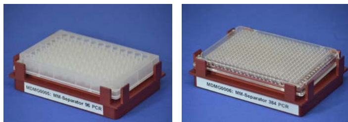
Fig 2. Magnetic Separators for 96 and 384 well PCR plates for automated processing (MDMG0005 and MDMG0006)
